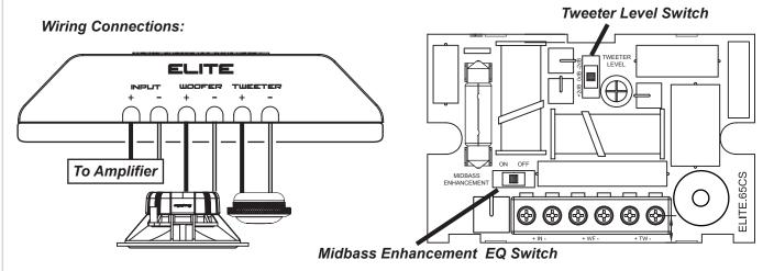
**Tweeter Protection:** Most component speakers offer a simple one stage "tweeter shut down" for protection. The Elite system provides two stages (polyswitch and lightbulb) that variably optimizes the signal to the tweeter when automatically activated. This protection system adapts to the dynamic signal level of the music, so it always provides just the "right" level of protection.
